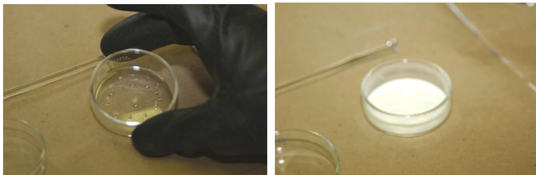
Figure 3: Real Agent Testing at Battelle: Agent on the Petri Dish (Left) and Agent with FAST-ACT (Right)
